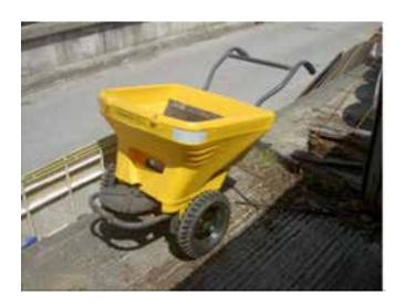
WSCC recommends a spread rate of approximately 20 grams of salt/grit per metres square when hand salting. Although salt/grit can be spread effectively with shovels, care is required to ensure over salting does not occur. Push-along devices, as shown on the left, can be used to cover large areas with an even spread. Large areas can thus quicker treated with wastage.
