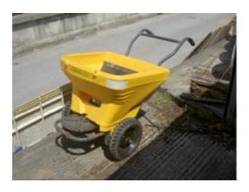
WSCC recommends a spread rate of approximately 20 grams of salt/grit per metres square when hand salting. Although salt/grit can be spread effectively with shovels, care is required to ensure over salting not occur. Push-along does devices, as shown on the left, can be used to cover large areas with an even spread. Large areas can thus be treated quicker with less wastage.
