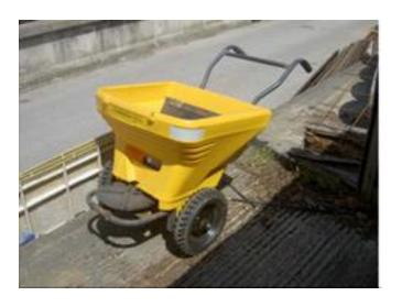
WSCC recommends a spread rate of approximately 20 grams of salt/grit per metres square when hand salting. Although salt/grit can be spread effectively with shovels, care is required to ensure over salting not occur. Push-along does devices, as shown on the left, can be used to cover large areas with an even spread. Large areas can thus be treated auicker with less wastage.
