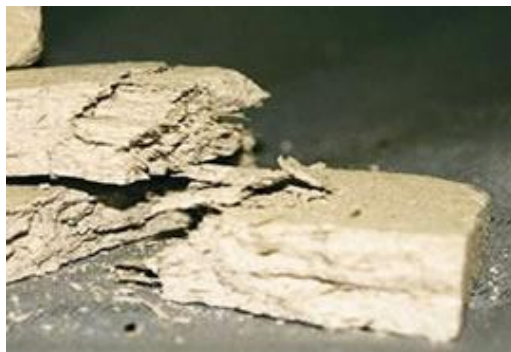
Pieces of Asbestos Insulating Board (AIB)
