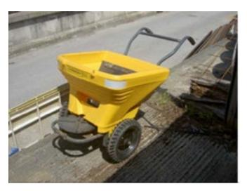
WSCC recommends a spread rate of approximately 20 grams of salt/grit per metres square when hand salting. Although salt/grit can be spread effectively with shovels, care is required to ensure over salting does not occur. Push-along devices, as shown on the left, can be used to cover large areas with an even spread. Large areas can thus be treated quicker with less wastage.
